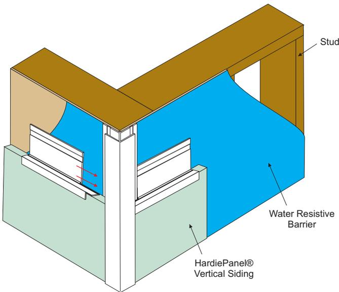
**MATERIAL:** Custom die-extruded from heavy-duty, 6063 T-5 extruded aluminum.
