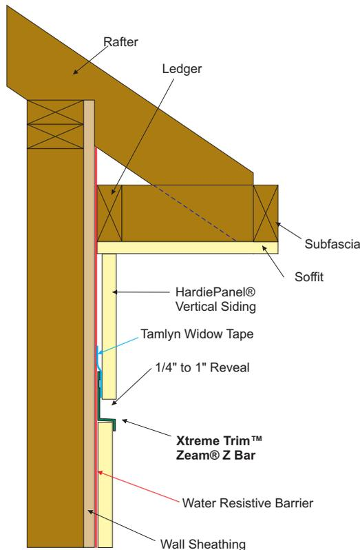
**MATERIAL:** Custom die-extruded from heavy-duty, 6063 T-5 extruded aluminum.
