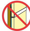
**Do not install J Mold on Horizontal applications where the exterior flange can catch water. J Mold should not be used on the top header of doors or windows.**
