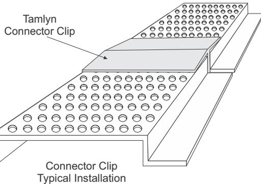
**MATERIAL:** Extruded rigid PVC, industry-standard, durable, chemically resistant product designed for outdoor weatherability.
